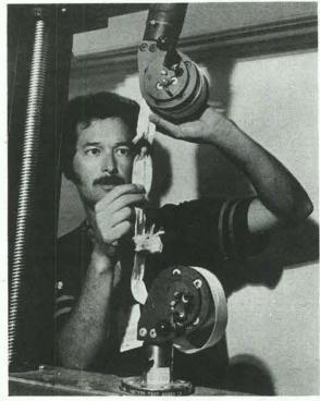
BREAKING POINT of parachute material is determined on this machine by Ken Ronquillo. Goal in chute development is maximum strength, minimum volume because space available is always limited.
